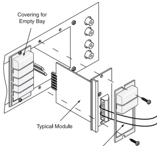
Feed wires through cover before making connections.
