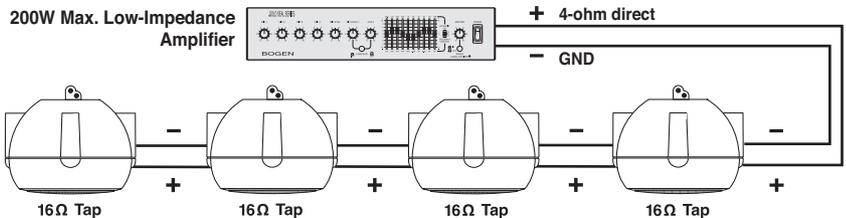
**EXAMPLE:** Four 16-ohm speakers in parallel = 4 ohms. Also in this example, the amplifier output power rating capability should not exceed 200W (4 X 50W, the MPS1/2).
