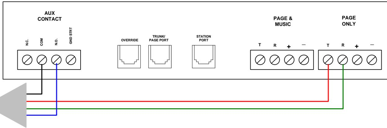
The DFT120 is designed to accept a Loop Start, Page Port, or a Page Port .
