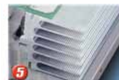
Two Custom Extruded Heat Sinks Provide Heat Transfer from Output Transistors
