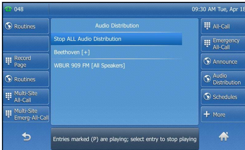
Figure 130. NQ-T1100 Admin Phone Audio Distribution Display
